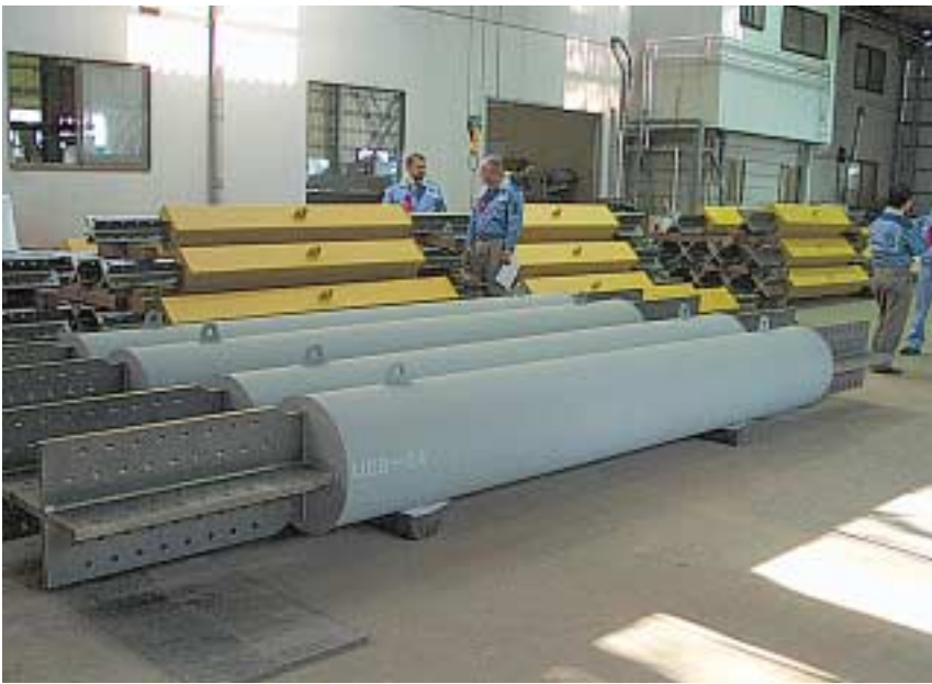
Fig. 5. Unbonded braces at fabrication plant, Chino, Japan.
